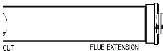
Offset Flue L = 4 m Max plus 2 bend 90° and Combi ridge
